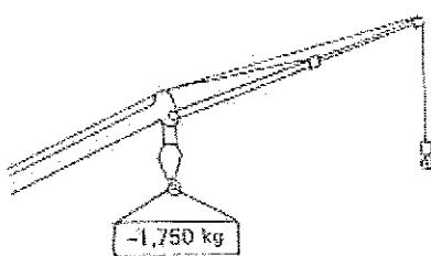
7. Tip over angles at each boom are as given in the right table. Don't reduce boom angles smaller than given therein.
