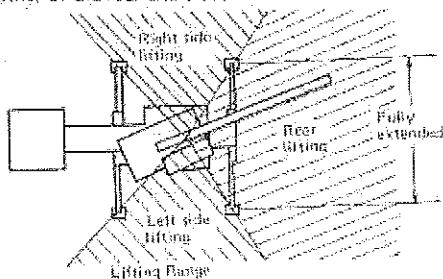
4. The rated lifting capacities for operation without outriggers is based on best condition of the tire air pressure and the ground surface.
